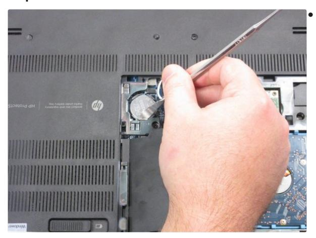
Use a plastic or metal spudger to release the CMOS battery from the clips.
