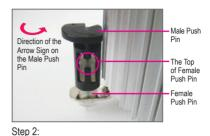
Before installing the cooler, note the direction of the arrow sign on the male push pin. (Turning the push pin along the direction of arrow is to remove the cooler, on the contrary, is to install.)
