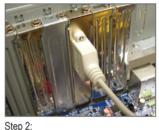
Secure the metal bracket to the chassis back panel with a screw.
