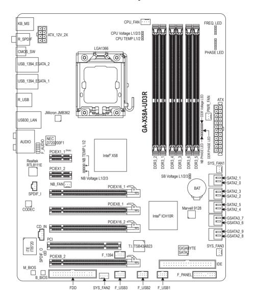
(Note) Due to a hardware limitation, the PCIEX1\_1 slot can only accommodate a shorter PCI Express x1 expansion card. For a longer expansion card, use other expansion slots.
